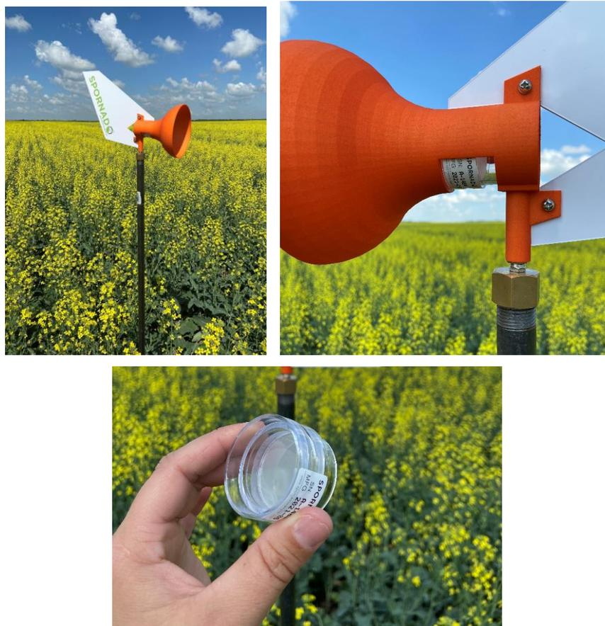
Figure 1. Spornado spore sampler installation and cassette insertion.
